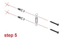
Move the cabinet to its final position on the wall and mark the location of the second bracket (A) on the wall. For concrete walls, drill holes and insert the plugs (B).
