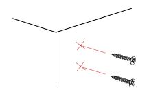
Attach one bracket (A) to the backside of the cabinet just below the top edge of the cabinet by using the screws (D).
