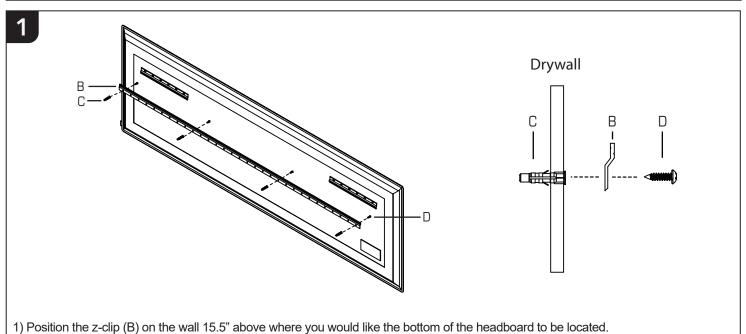
Use a level to ensure the z-clip (B) is level and secure with 4-6 provided screws. If attaching to drywall use supplied anchors (C).
