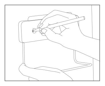
Place bracket onto door and lightly mark position of screw holes with a pencil.
