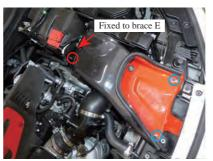
33. Fix the two front parts of the introduction duct with the original bolts. Fix the rear side to brace E while adjusting the position. (Using screw Bx1)
