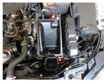
5. Remove the two bolts and remove the bottom of the box.
