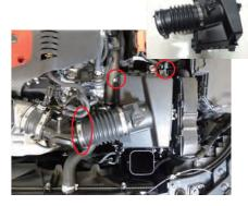
3. Loosen the hose band, remove the two clips. and remove the top of the box.
