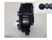
6. Remove the three rubber bushes from the bottom of the box
