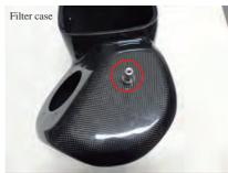
15. Attach the aluminum stud to the filter case. (Using Bolt Cx1)
