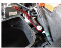
29. Fix brace E on top of brace A of the filter case using the original bolt.
