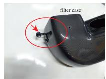
12. Attach the rubber bushing removed from the original filter box to brace A. Then attach brace A to the filter case. (Using 1 bolt A and 1 nut)
