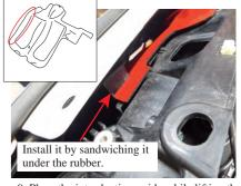
9. Place the introduction guide while lifting the bumper. Place the original rubber guide on top of the red circle and widen the opening.
