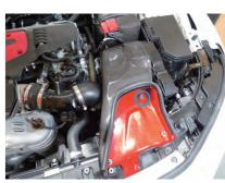
32. Place the introduction duct ASSY over the filter case and insert the rubber bushing into the aluminum stud.
