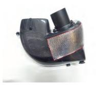
22. Attach the heat-resistant mat referring to the diagram above.
