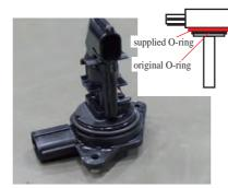
18. Attach the supplied O-ring to the air mass sensor by placing it on top of the original O-ring.
