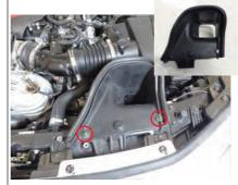
1. Loosen the two bolts and remove the introduction duct.
