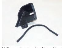
11. Temporarily remove the rubber molding of the introduction duct. (Please leave the pin in place)
