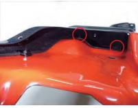
24. Assemble the introduction plate and introduction cover. Insert the bolt Ax2 from above and fix it with the nut x2.
