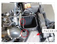
31. Attach the intermediate clamp of the air mass sensor wiring to brace B. Then install the sensor coupler.
