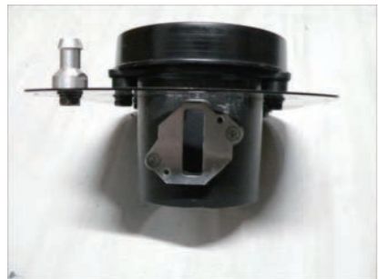
19. Install conversion plate with bolt E (tapered).
