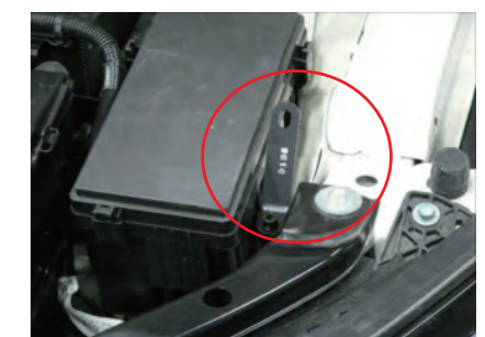
12. Place the 20 mm spacer under brace B(0135) and secure it using bolt C.
