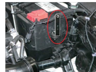
11. Attach brace A(0028) on the rubber stud bolt with the nut in the direction circled in red.
