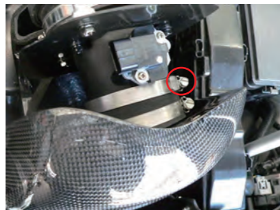
23. Connect the sensor adapter assembly to the hose. Temporarily tighten the hose band so that it turns a little.
