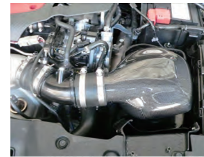
29. Re-install the intake chamber assembly again and tighten the hose band.
