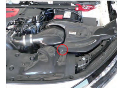
35. Secure the side introduction duct to the front introduction duct using bolt D.
