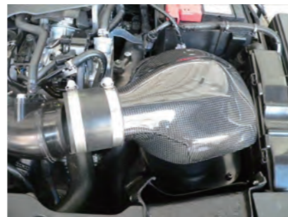
24. Place the chamber assembly in the filter box once to orient the chamber.
