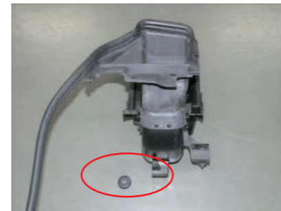
4. Remove the grommet from the bottom of the box.
