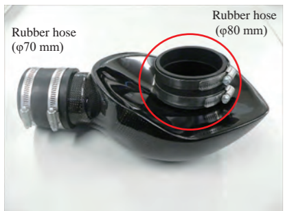
22. Attach a rubber hose to each end of the chamber as shown. Insert the \phi 80 hose all the way back and temporarily tighten with band #56. Place the head of the screw on the hose band in the same direction as shown.
