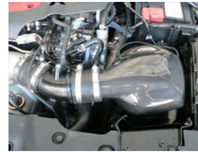
25. Orient the chamber so that the two aluminum studs in the plate firmly pierce the O-ring grommet on the filter box.
