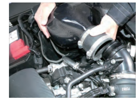
27. Remove the chamber assembly once. Lift the chamber and fixation plate together and remove.
