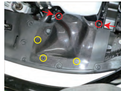
31. Attach the front introduction duct. Red : Bolt D Yellow : Clip
