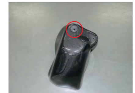
9. Port the original grommet removed in step 4.
