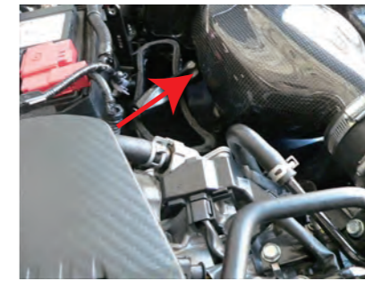
26. Completely tighten the hose band in the direction indicated by the red arrow once the chamber is properly fitted.
