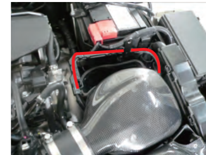
32. Route the air mass sensor wiring as indicated by the red line and secure it with a zip tie.
