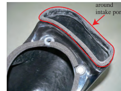
8. Attach the thin sponge tape around intake port as shown.
