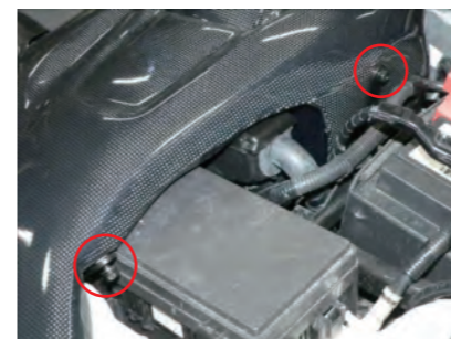
34. Secure the side introduction duct to the filter box from above and secure it to the brace with bolt A.
