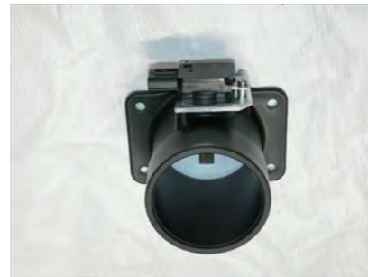
18. Insert an M4 spacer between the sensor adapter and the sensor, and attach with bolt E.
