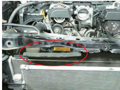
13. Fold the sponge attached on top of the radiator forward.
