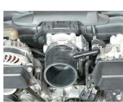
24. Insert the nipple in the silicone hose as shown and secure it with a hose band.
