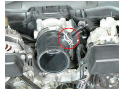
25. Remove the OEM hose band of the blow-by hose and replace it with the supplied hose band. Secure the nipple with an insert band.
