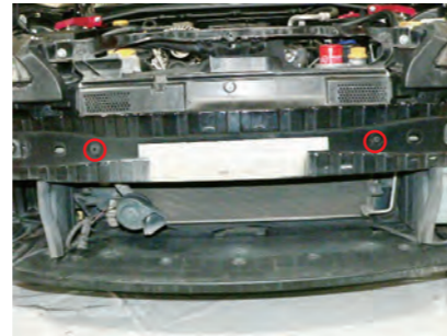
15. Install the M5 well nut and M4 well nut to the front member as shown in red.
