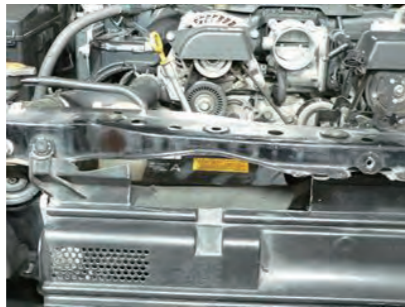
14. Install the panel with the OEM clips by sandwiching the bent sponge.
