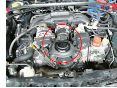
26. Attach the adapter ASSY to the silicone hose. Loosely attach the hose band. DO NOT Tighten.
