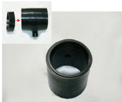
22. Put a rubber ring inside the long side of the silicone hose as soon.
