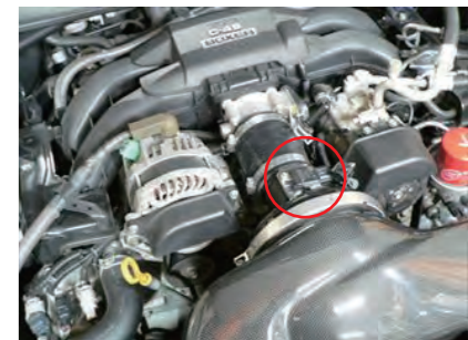
33. Reconnect wiring to mass air flow sensor. Tighten the hose band on the sensor adapter side. (Be careful not to let the wiring interfere with the pulley.)
