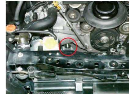
27. Put 2 washers on the top and bottom of the rubber stud bolt shown in red and attach it to the body.
