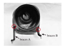
12. Temporarily fasten each brace to the chamber box with bolt A in two places.
