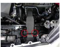
1. Remove the two clips and remove the introduction duct.
