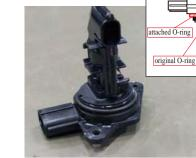
8. Install the attached O-ring on the air mass sensor, over the factory O-ring as illustrated in red.
