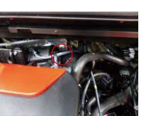
4. Remove the vacuum hose. Attach the attached rubber cap to the removed part.
