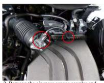
2. Remove the air mass sensor coupler and remove the wiring clip from the filter box.
