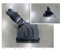
6. Loosen the hose band, remove the suction hose from the filter box, and remove the air mass sensor from the filter box.
