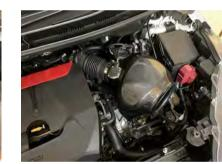
15. Tighten each brace. Tighten the hose band. Install the air mass sensor coupler and secure the wiring with tie wraps.
