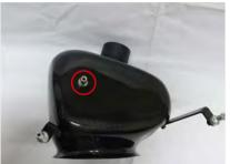
13. Attach the aluminum stud to the chamber box with bolt B.
