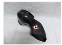
17. Install the grommet on the back of the air duct.
