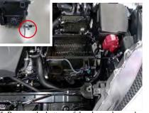
5. Remove the bottom of the cleaner box and remove the actuator from the filter box
