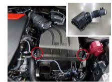
3. Loosen the suction hose band and remove the upper part of the factory filter box and the intake hose.
