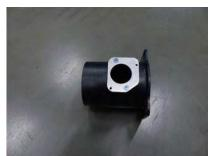
7. Attach the adapter plate to the sensor housing with 2 countersunk screws. Pay attention to the orientation of the conversion plate.
