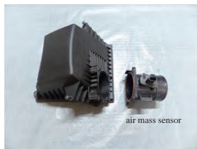
5. Remove the air mass sensor by loosening the four bolts from the top of the box.
