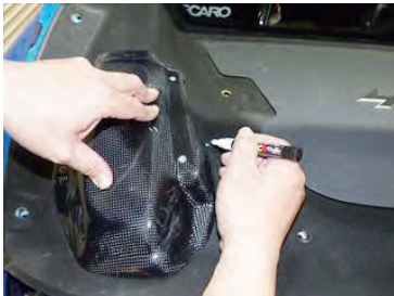
(4) Mark the semicircular part on the front side of the panel (S).
