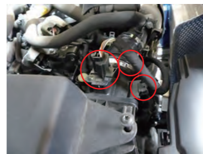
3. Remove the wire clamp and sensor coupler and loosen the suction hose band.
