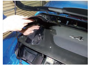
(3) Remove the carbon panel (L) while holding down the carbon panel (S).
