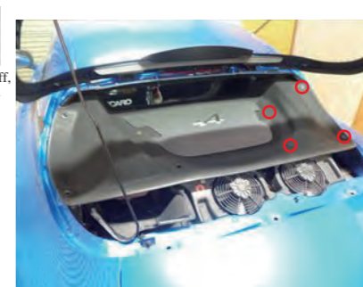
17. Attach the engine cover to the vehicle and fix the red circle mark with the original bolt.
