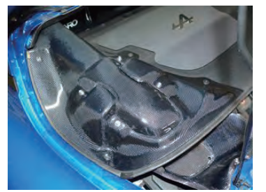
(13) Attach the engine cover and carbon panels (L) and (S) to complete the work.
