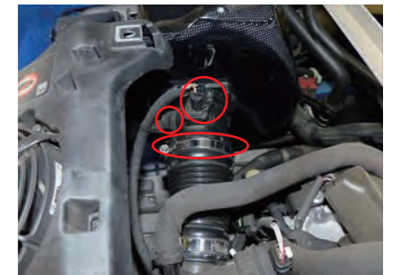
12. Install the wire clamp and sensor coupler, and tighten the suction hose band.
