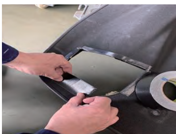
(11) Finish the cut section with tape or the like.
