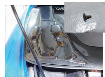
18. Fix the carbon panels (L) and (S) using the 4 genuine bolts that were disassembled. (Use only bolts, not washers)
