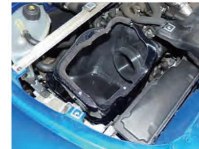
10. Remove the carbon scoop and place the carbon case in the engine room.
