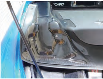
(1) Install up to the carbon panel once in the same way up to step 18 of the instruction manual. We will mark the cut line to cut the engine cover.
