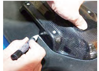
(5) Mark the line on the engine cover so that it does not shift.
