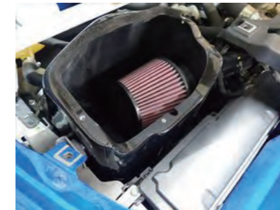
13. Attach the filter to the funnel adapter and tighten the hose band.
