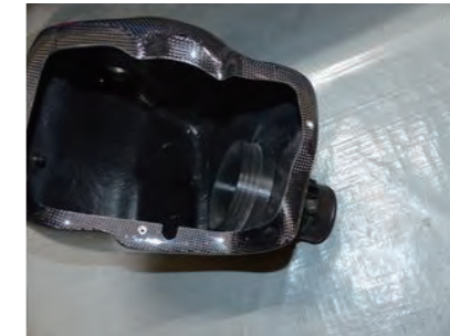
8. Insert the funnel adapter into the case and fix the air mass sensor from the outside of the case with 4 bolts (A).
