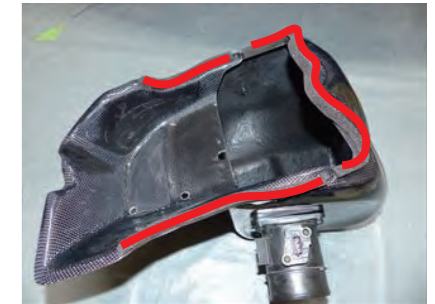
9. Fix the carbon scoop and the carbon case with bolts (C) x3, and paste the sponge tape on the red line in the above figure.
