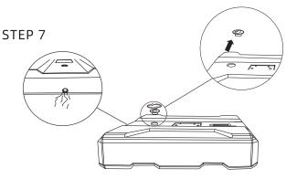
You could open up the drain lid to drain the water inside when not in use.
