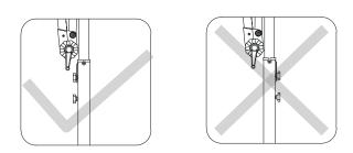
NOTE: Make sure the two knobs and the crank are on the same side
