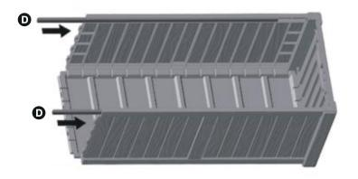
Insert two iron rods (Part D) into the top of two Part A.
