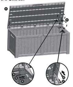
Use 5 screws for each side to install each pressure bar on Part C and Part J
