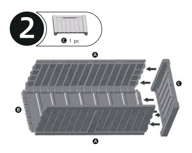
Only Insert one Part C to Parts A and B. DO NOT insert another Part C in this step!
