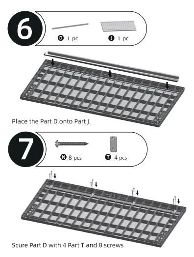
This step prevents the lid from bending causing by the sun exposure and temperature variation.
