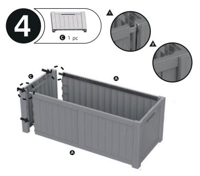
So far you have one Part C left. Go ahead and install it to Parts A and B
