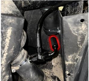
2. The Female fitting will be connected to the fuel line from the fuel pump.
