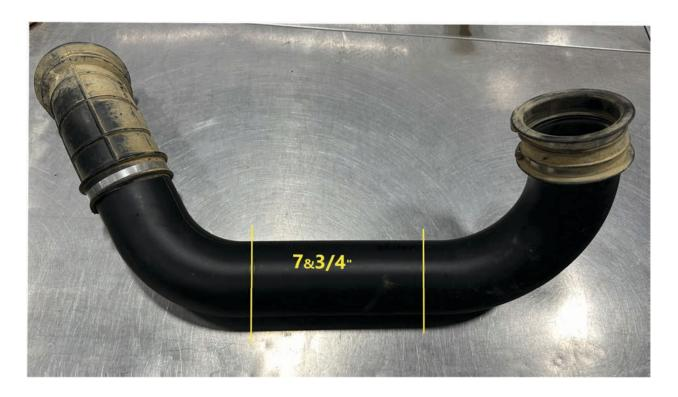
**#3** With the section cut out & removed, install the silicone onto the fan with clamps, and then the silicone onto the factory plastic tube with clamps in place. Soap & water applied to the surfaces allows for easy installation and movement of the silicone. Do not tighten the clamps at this time.
