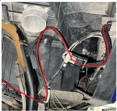
The clutch fan will be pulling fresh air in from the bed intake, pushing it into the clutch housing, while forcing hot air out of the exit ducts of the clutch. The fan will run anytime the tail light is on, the machine does not need to be running for the fan to be on.
