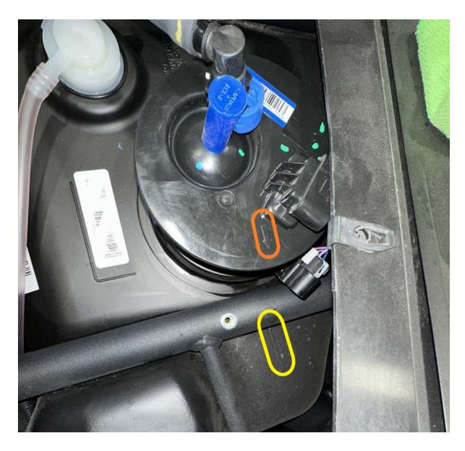
**#8** Install fuel line and wiring plug being sure to re-clip the gray portion of the electrical plug and blue clip of the fuel line.
