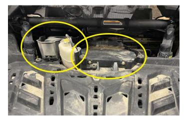
2. Remove the clamp of the charge tube at the throttle body.
