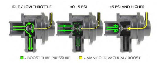
The X3's should have some blow off during idle and cruising speeds. Trying to keep the valve closed with a extremely heavy spring builds heat in the charge tube from pushing air on the backside of the essentially closed throttle blade.
