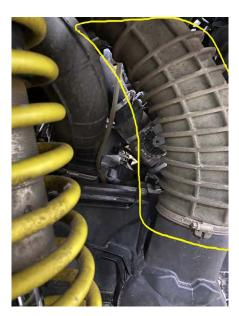
And remove the air intake, and what would normally be the intercooler cover.
