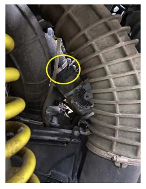
3. Remove the clamp of the charge tube at the cold side of the turbo.
