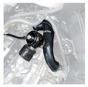
5. Adjust the tube so that the fitment is correct, tighten the turbo side first, followed by the throttle body side.
