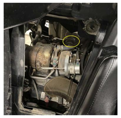
4. With the factory charge tube and clamps removed you can slide the clamps onto your RPM charge tube and begin to install the tube between the turbo and throttle body.
