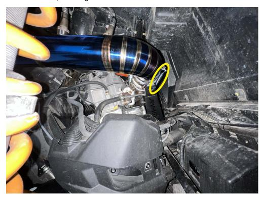
\*\*\* **3" Titanium E-Valve** After first Full Heat Cycle re-torque the steel clamping nut to 65(lb-ft).
