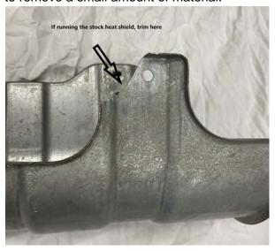
If using the 2nd O2 bung on the 2.5" E-Valve Exhaust, you may need to trim the heat shield to allow room for the 2nd O2 bung.
