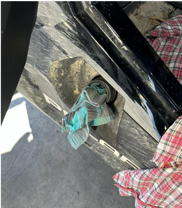
**Using a  $\frac{1}{2}$ " drill bit, drill the hole slowly.**
