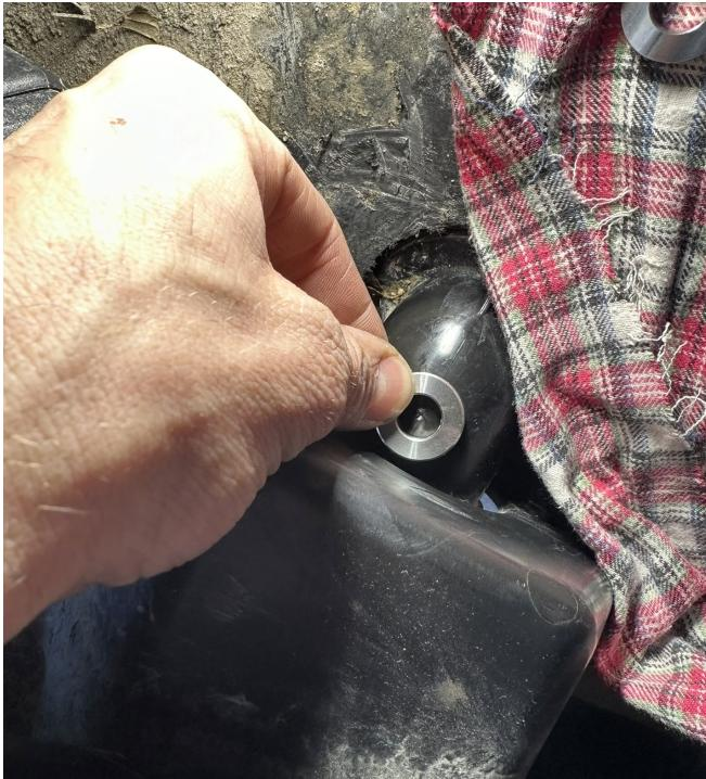
**Remove the gas cap and stuff a rag into the fill neck to catch any debris.**
