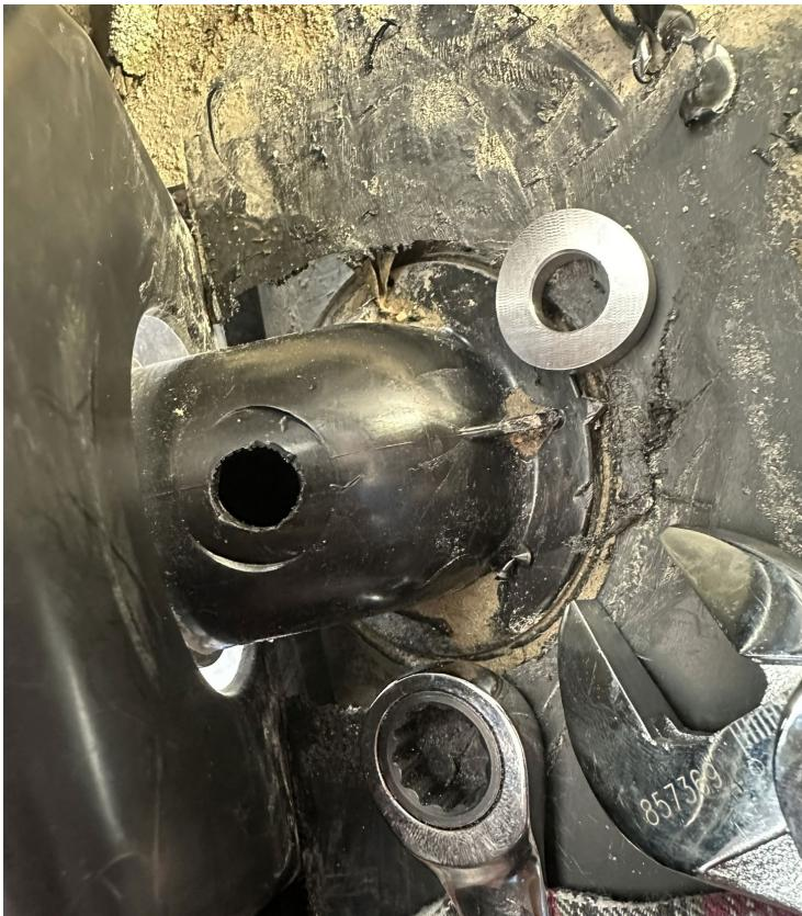
Apply Loctite to the threads & install the fitting. Be sure that the curvatures of the outside and inside washers remain in line with the curvature of the fill neck. The pressure of the stainless washer will seal the unit. Over tightening can result in splitting the plastic resulting in needing the gas tank replaced! Once tight, align the nut with a pin hole and insert the Cotter Pin and bend both ends to secure.
