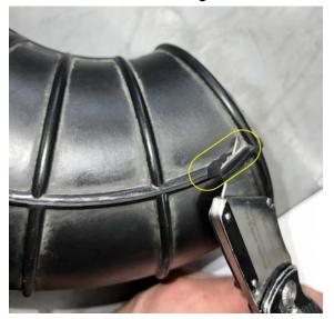
4. Slide the t-bolt clamps onto the tube and apply soapy water to the inside of the tube and clamping area of the ECF. Firmly push the ECF into the rubber tube.
