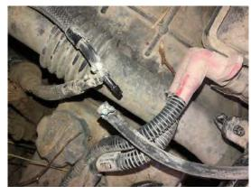
**5.** Install tnew vacuum line hose provided in the kit between the T and diverter valve. (CA models will need to modify/extend the stock vacuum line)
