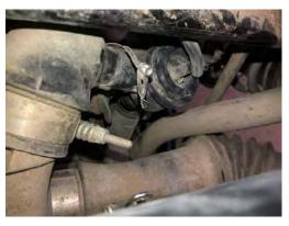
1. Locate the original diverter valve. It is located on the drivers side of the machine and can be accessed through the engine access cover and drives side rear shock.
