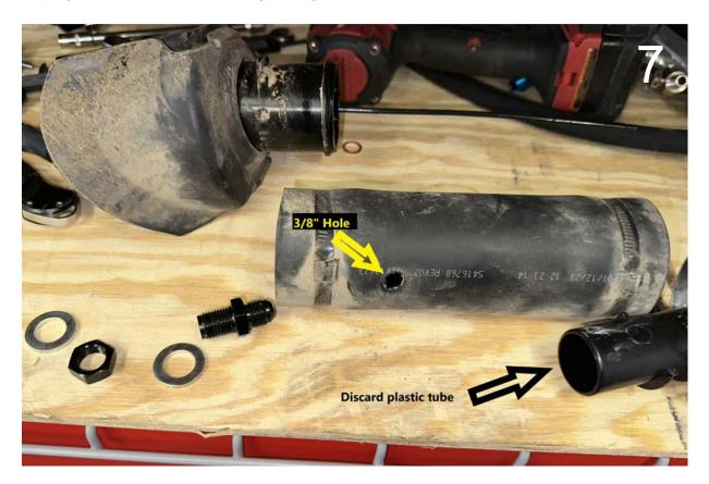
22. At this time you can secure the stainless fitting, use loctite and make sure both sealing washers are in place. Install the -6an 90\* fitting to the bulkhead.
