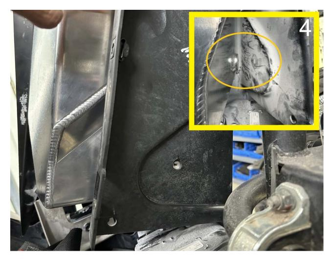
9. At this time you can remove the bolts, apply loctite, and begin to tighten all mounting points evenly and in random order.
