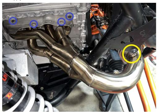
16. Wipe the entire header pipe clean of and oils from handling the pipe in order to prevent stains once heated up.
