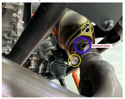
3. Unplug the O2 sensor from the harness and remove it from the exhaust pipe. .
