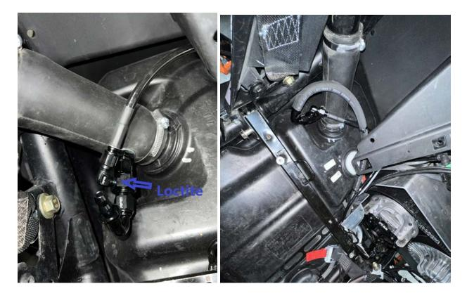
At this time you will move to the wiring of the fuel pump. Secure the Red to the + and black to the -. Secure the wiring using a zip tie to the fitting above as pictured.
