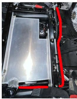
With all the lines secured to the bulkhead fitting it's a good idea to secure all the hoses to the square tube, away from the clutch cover.
