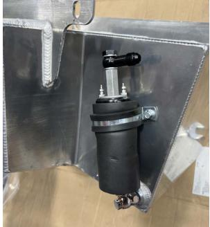
With the fuel pump assembly installed onto the tank, you can install the fuel tank into place.
