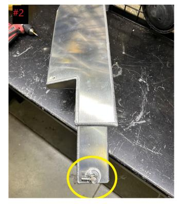
4. Attach the -6an hose to the barb and route it to the right & behind the frame rail as pictured. See Picture #3. This is important that the fuel line remains on the right side and behind the frame rail during and after installation. ( Use heat to soften the -6an line before pressing it onto the barb fittings for easier installation ) See Picture #3
