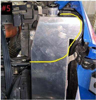
8. Begin to route the -6an and -4an lines on the frame rail as pictured. All lines should be on the back side when possible, and away from the sway bar. Secure the lines using the supplied zip ties. Be sure the lines clear the firewall cover. See image #6
