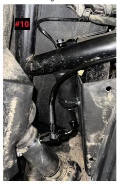
13. Attach the 90\* -4an fitting ( use loctite ) to the fitting as pictured with a slight upward and forward angle allowing the -4an line to easily attach to it. At this time the fittings should all still remain loose. With these fittings in place, you can now mark on the rubber fill tube where the hole needs to be for the bulkhead fitting. See Image #10 WIRING HARNESS SIDE OF PUMP IS AT THE BOTTOM
