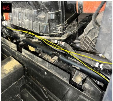
9. Assemble 1 stainless barb and 1 90\* -6an fittings using a 2" piece of the supplied -6an line.
