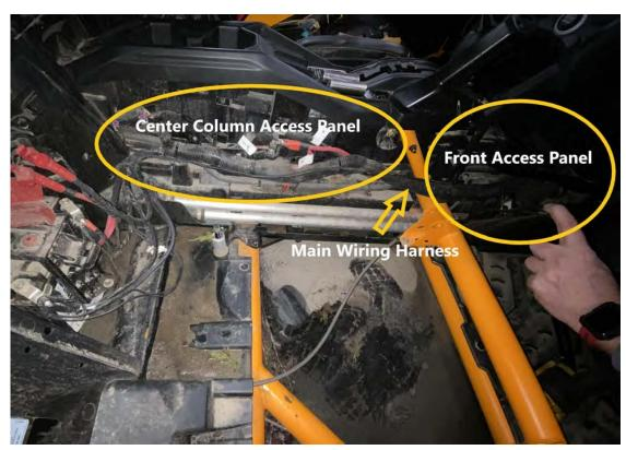
**#2** Route the switch side of the harness to the prefered toggle location. Push the harness and plug through the back side, then install the switch. With the switch plugged into the harness you may now push the switch into place.
