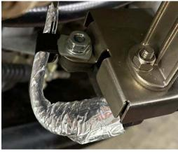
**#7** Our harness is built to suit 2 and 4 seat Maverick R's. Any extra slack can be coiled, and secured behind the center console access panel neatly and securely. Carefully check all wiring and securing any spots where there is slack.
