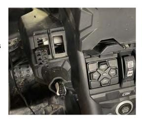
**3.3** Remove the cover to the buss bar gaining access to your positive and negative terminals. Red goes on the bottom 12v keyed ignition terminal, and black to the top ground terminal. At this time you can verify you have a 10amp mini bus fuse installed in the fuse holder. With the wires. Place the busbar cover back on the busbar.
