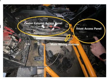
**3.2** Route the switch side of the harness to the prefered toggle location. Push the harness and plug through the back side, then install the switch. With the switch plugged into the harness you may now push the switch into place.
