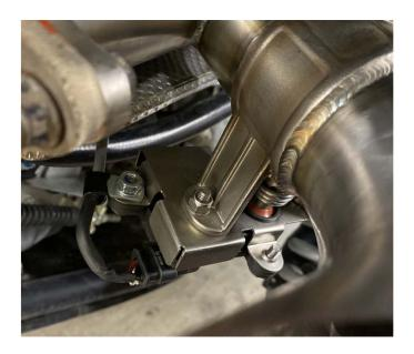
**3.6** Our harness is built to suit 2 and 4 seat Maverick R's. Any extra slack can be coiled, and secured behind the center console access panel neatly and securely. Carefully check all wiring and securing any spots where there is slack.
