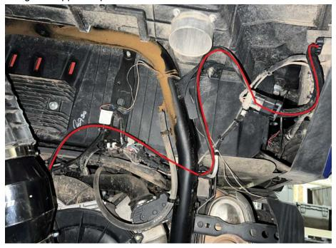
6. At this time you can verify everything is tight, securely fastened, and turn the machine on. You will hear the fan fire up. The fan intakes fresh air through the bed box, and forces it into the clutch housing. This blows cool dry air across the clutches.
