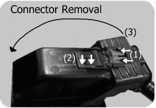
**STEP 4** – The ECM is secured in its cradle by two large plastic tabs on the top of the ECM. With your thumbs, push up on each tab while pulling the ECM towards the rear of the vehicle. Once both tabs are released, the ECM is now free of the vehicle and may be pulled out of the wheel well.
