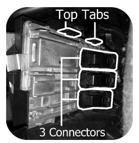
Press each of the three ECM connectors back into the ECM, close the connector clamps until they click into place, then slide in the red locking tabs.
