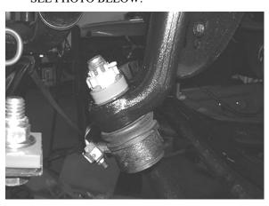
26. Locate the supplied FT30205 stabilizer bracket and install it in the factory location using the original hardware and torque to 65 ft. lbs. Re-connect the stabilizer to the new drop bracket and tighten to 45lbs. SEE PHOTO BEOLW.
