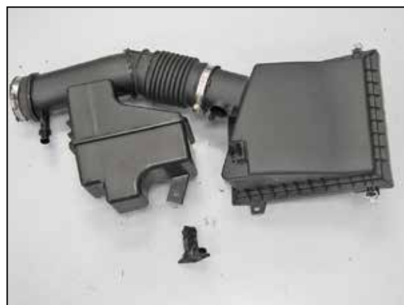
15. Remove the mass air sensor from the factory air filter housing.
