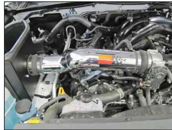
18. Install the intake tube into the coupling hose at the throttle body and then into the coupling at the filter adapter. Adjust the tube for best fit and then secure with the provided hose clamps.
