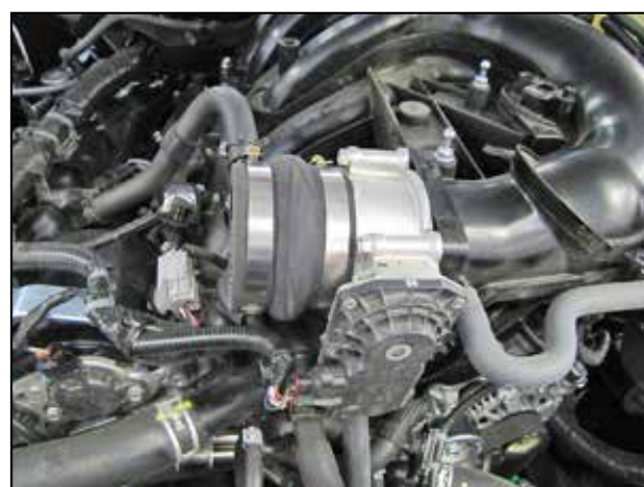
13. Install the provided hump coupler (08171) onto the throttle body and secure with the provided hose clamp.
