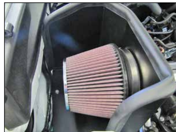
21. Install the K&N® air filter onto the filter adapter and secure with the provided hose clamp. NOTE: Drycharger® air filter wrap; part # 22-8049DK is available to purchase separately. To learn more about Drycharger® filter wraps or look up color availability please visit http://www.knfilters.com .
