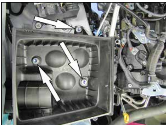
7. Remove the three bolts securing the lower air filter housing to the inner fender and then remove the lower air filter housing from the vehicle. NOTE: K&N Engineering, Inc., recommends that customers do not discard factory air intake.
