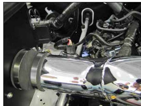
20. Reconnect the mass air sensor electrical connection.
