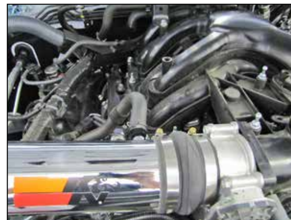
19. Connect the crank case vent fitting onto the vent fitting installed into the K&N® intake tube.
