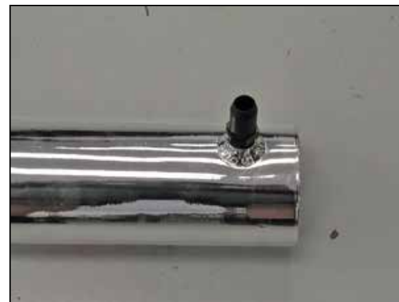
17. Install the provided vent fitting into the K&N® intake tube as shown. NOTE: Plastic NPT fittings are easy to cross thread. Install the vent fitting “hand” tight, then turn it two complete turns with a wrench.
