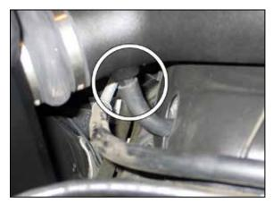
26. Connect the crank case vent hose to the vent fitting installed into the K&N® intake tube. Secure with the provided hose clamp.
