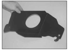
11. Install the "L" bracket (070812) onto the rear of the heat shield as shown with the provided hardware.
