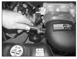
20. Install the supplied vent hose onto the vent port on the valve cover and secure with the provided hose clamp, then onto the K&N® intake tube as shown.
