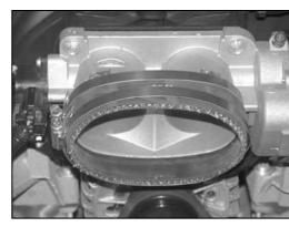
18. Install the silicone hose (08541) onto the throttle body with the provided hose clamps as shown.
