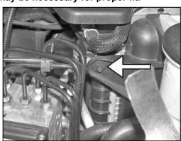
14. Remove the radiator fan shroud mounting bolt shown.
