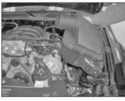
6. Remove the air box assembly as shown. NOTE: K&N Engineering, Inc., recommends that customers do not discard factory air intake.
