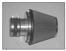
24. Install the air filter onto the air filter adapter and secure with the provided hose clamp as shown.
