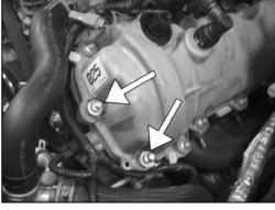
8. Remove the two valve cover bolts shown. NOTE: These bolts will be reused.
