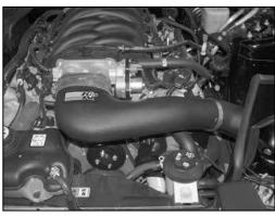
19. Install the K&N® intake tube into the silicone hose at the throttle body and onto the saddle bracket assembly then secure with the provided hose clamps as shown.
