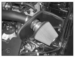
25. Install the air filter assembly onto the K&N® intake tube as shown and secure with the provided hose clamp.
