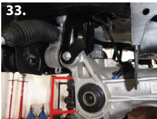
31. Install differential into drop brackets using provided hardware. (pic 33)
