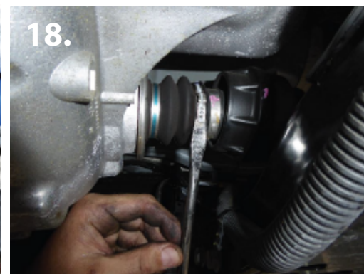
17. Remove bolts from factory front driveline. You will not re-use the bolts. (pic 17) 18. Remove boot retainer clip. You will not re-use. (pic 18) 19. Remove factory front driveline. (pic 19)
