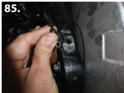
75. Attach brake sensor wire on driver side spindle. Factory tab DOES NOT go into hole on spindle. (pic 84)
