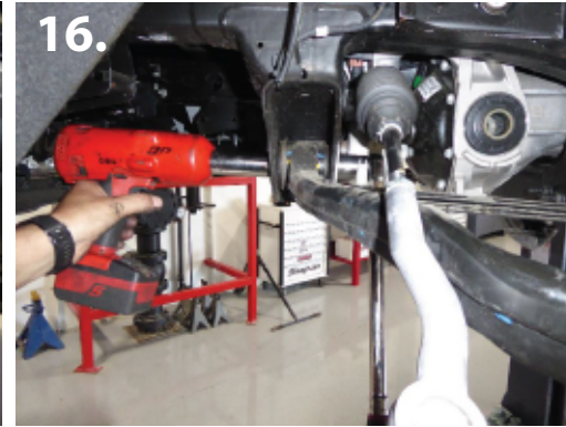
15. Remove factory skid plate. (13mm) (pic 15) 16. Remove factory lower control arm. (27mm) (pic 16)
