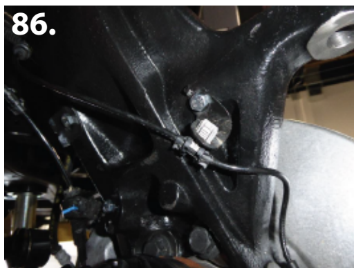
75. Attach brake sensor wire on driver side spindle. Factory tab DOES NOT go into hole on spindle. (pic 84)
