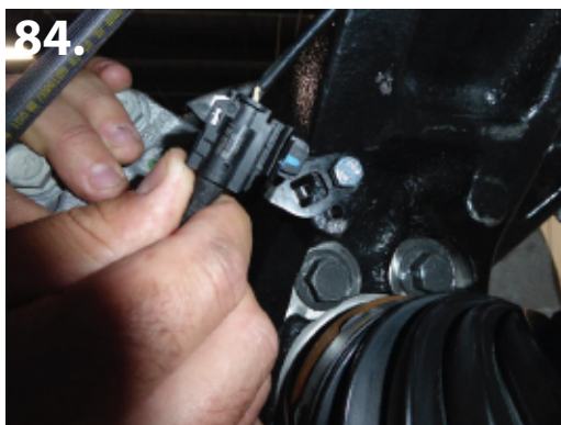
75. Attach brake sensor wire on driver side spindle. Factory tab DOES NOT go into hole on spindle. (pic 84)
