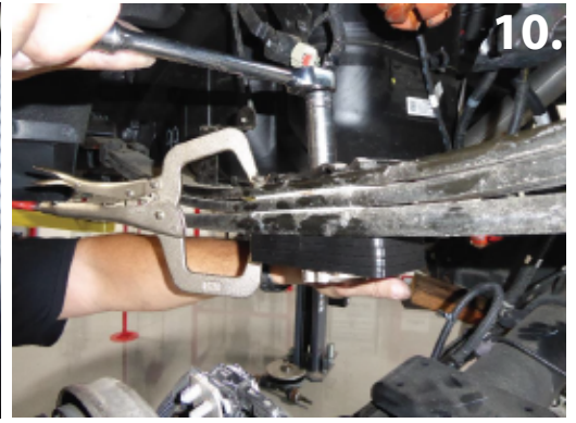
9. If your vehicle has a tapered shim under leafs, you must remove that shim. Clamp leaf pack together and remove center pin. Remove the tapered shim. (pic 9-10)
