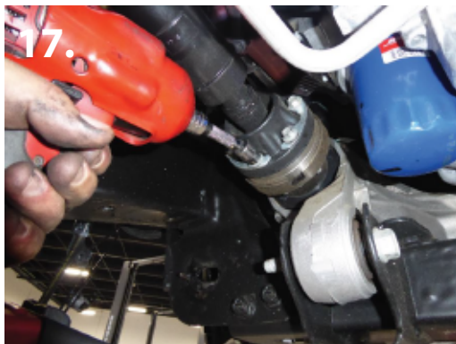
17. Remove bolts from factory front driveline. You will not re-use the bolts. (pic 17) 18. Remove boot retainer clip. You will not re-use. (pic 18) 19. Remove factory front driveline. (pic 19)
