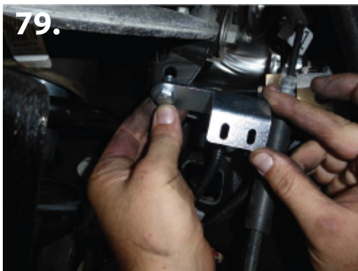
71. Install new abs sensor drop bracket located inside the hardware bag. (pic 79-80)
