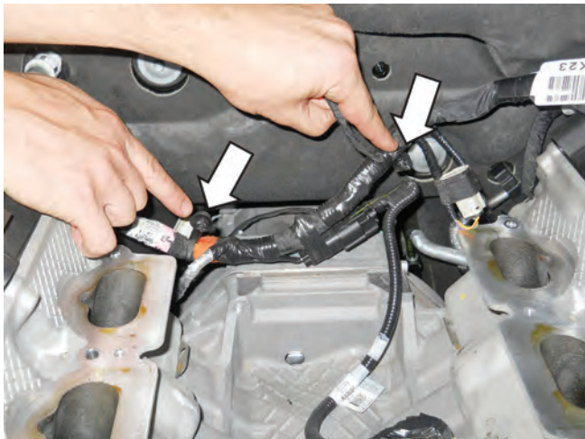
Pin retainers on harness
