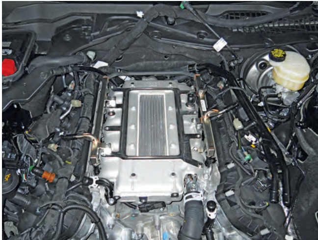
14. Connect the eight (8) fuel injector electrical connectors.
