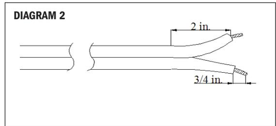
NOTE: Using the correct gauge cable is essential for obtaining proper lighting performance. For use with SPT-3, SPT-2W, underground low energy circuit outdoor type cable (Minimum 25' length).
