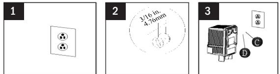
NOTE: Do not attach the transformer to the wall at this time. First, connect the low voltage cable to the transformer terminals.
