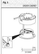
1) TURN OFF ALL ELECTRICAL POWER BEFORE INSTALLING. REMOVE RING SOCKET FROM PUCKLIGHT IF NECESSARY, CONNECT WRP8----- OR SIMILAR CABLE TO PUSH IN CONNECTOR.
