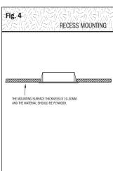
3) THREAD THE WIRE THROUGH THE CABINET HOLE. 4) PUSH PUCKLIGHT INTO THE HOLE.
