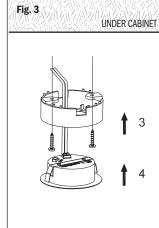
3) SCREW IN THE RING SOCKET TO THE MOUNTING SURFACE. THREAD THE WIRE THROUGH THE CABINET HOLE (MAKE 3/5" HOLE UNDER CABINET) PRESS IN THE PUCKLIGHT TO THE SOCKET.
