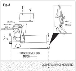
2) SCREW IN THE TRANSFORM BOX THE MOUNTING SURFACE, THAN, UN SCREW THE LID AND CONNECT 120V AC CABLE TO LUMINIZ TRANSFORMER BOX BY USING THE OUICK CONNECTORS.
