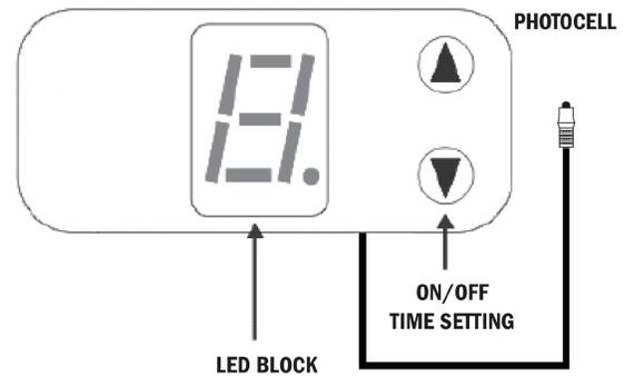
The photo cell operates with a slight time delay to prevent false reactions to momentary changes in ambient light conditions, such as car headlights.
