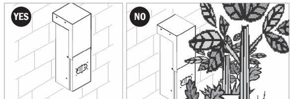
Keep transformer free from any obstructions. This will prevent the photo cell from turning the system "ON" prematurely.
