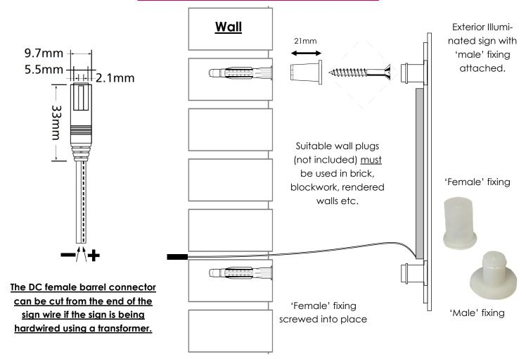
Using a scrap sheet of cardboard or paper and a soft under surface, push your sign (fixing points facing down) into the paper to form indents. Or carefully measure the holes centres from the small points on the male fixings.
