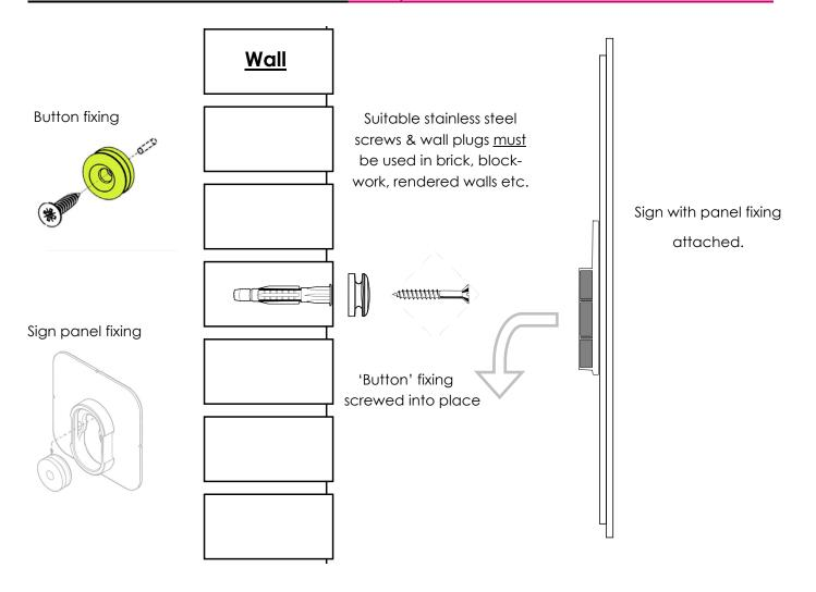
Carefully measure the hole centres using the sign back.
