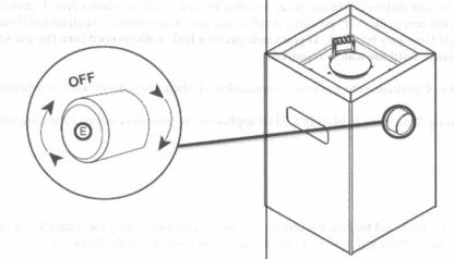
2. To attach the gas tank into the fire column, insert tank from bottom and screw into the regulator inlet fitting counter clockwise until hand tight.
