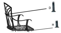
Seat (5) using 2xWashers and the wrench ..DO NOT over tighten.
