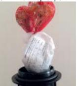
Remove 30g silica gel from the bag. Sign and date label. Place 30g silica gel into closure and tie to the connector bundle. Replace silica gel each time the closure is opened. Silica gel changes from yellow to green to indicate it is to be replaced.
