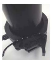
**15.** Place O ring bag into position. Apply clamp and close. Insert locking pin.
