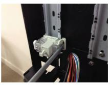
Take a flat headed screw driver and insert in to clasp located to the back side of the ECM 1B module. Exert an outward force whilst pushing down the module to engage and lock module into position on the indented din rail.
