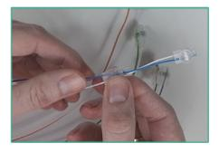
4. Slide the connector up to connector being replaced. The connectors should move freely along the wires.
