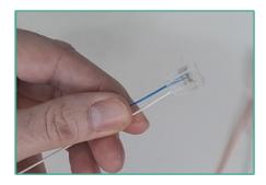
8. Confirm the connector is fully crimped and the flap is pushed in fully. The base should be fully pushed into the connector body. The 11A connector is in service.
