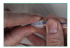
Insert the conductor wires from the side of the connector. Ensure the wires are pushed in fully.
