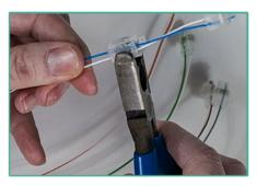
Using the approved crimping tool fully crimp the 11A connector.
