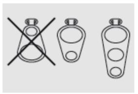
For branched configurations the sleeve must be positioned such that the adhesive flap and sleeve rails are over the largest cable (see illustration above)
