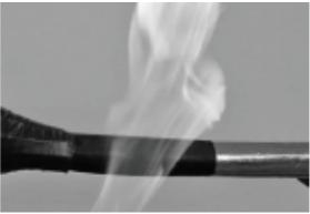
10. Preheat cable sheath sealing circumference using a blue flame. Brush flame for approx. 10 seconds. This removes any oxidants on the cable sheath.
