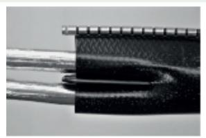
13. Position the sleeve centrally across the joint. Install all branch off clips as required. Ensure clips are totally inserted. The sleeve must be uniformally located around the cable diameter as shown above.
