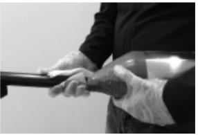
Remove cleaning tissue from its package and clean the cable for a distance of minimum 20cm at each end of the metal canister.
