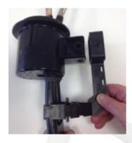
**7.** Attach the cable retainer on to the spigot on the closure base as shown.
