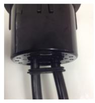
**5.** Clean cables again with PF Wet & Dry wipes. Insert cables into base using suitable size port size for the cable.
