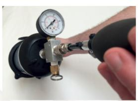
13. Pressure test using large dome tester and hand pump 30 minutes after sealant application. Recommend to pressure test all new closure installations using leak detection fluid at the base of the closure.
