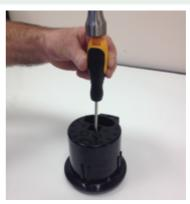
4. Choose the required size of the cable entry knockouts. Use appropriate size screw driver to knock out the hole. Ensure to turn the screwdriver to remove any sharp edges on the hole that has been punched.
