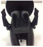
**11.** Seal cables to base of closure using putty to create a dam to prevent sealant from leaking.
