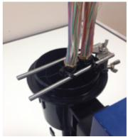
**10.** Remove O ring. Install cable jig as shown & finger tighten. Secure cables to jig with cable ties. Ensure cables are restrained and separated.
