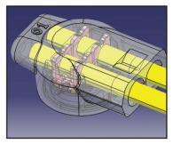
3. Fully insert wires fully into the connector base. The wires are visible in the base so you can see they inserted fully past the IDC blade contact. Precrimp if required using fingers if performing multiple crimping
