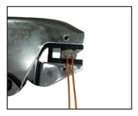
Use approved tooling for 2/3 wire connector terminations when installing. Apply pressure evenly to the top of the connector during crimping.
