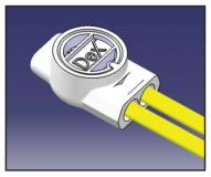
**5.** Fully crimp top cover so its flush with base housing top.
