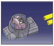
2. Ensure the wires to be terminated are cut flush and cleanly. Important no ragged edges are present on the insulation.
