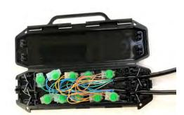
6. Evenly space the connectors in the gel filled splice chamber as shown. Push the connectors into the gel.
