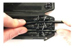
Press cable down firmly into the flapper area, as shown above.
