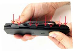
Push the top and base together and then push the latches over in the direction of the arrows.
