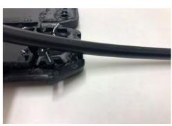
5. When installing the hard jacket 2/0.64 cable push in the cable from the edge of the closure in the direction of the flappers.
