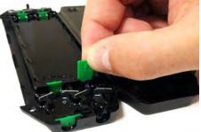
2. Remove inner and outer cable entry gates as required, as shown above. Only remove the gates where cables are being inserted. Use a pin nose pliers if required.
