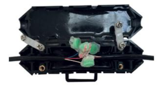
Insert 45mm of cable into each end of closure. Unscrew one side of each cable retainer & push cable into the slot. Leave 50mm of conductors for 8A connectors. Issue Date: 29/05/2015
