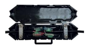
3. Position connectors in either side of the joint space. Screw cable retainers using a cross head screwdriver. It is important to screw down each side evenly to avoid cross threading. Screw down fully to allow the top gel filled compartment to close. Do not over tighten screws.
