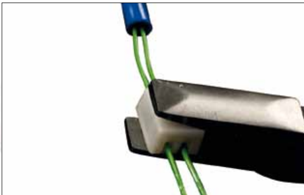
Crimping the connector and cutting wires.
